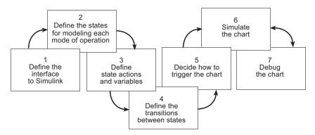
To get started quickly, you will participate in hands-on exercises that guide you through each phase of this workflow for building a realistic Stateflow chart and integrating it with a Simulink model. Note that work flows in one direction until you get to phase 6. At this phase, you may need to iterate between simulating and debugging your Stateflow chart as you fix errors and experiment with different parameters until the model produces the desired behavior.
