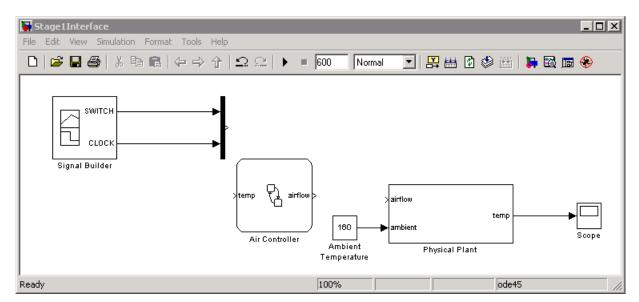
Notice that the input temp and output airflow have been added to the Stateflow block:
