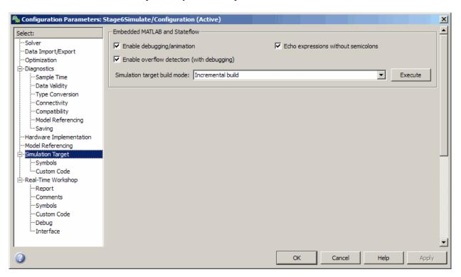
**Note** This dialog box is used to configure Stateflow software for building targets. A target is a program that executes a Stateflow chart or a Simulink model that contains a Stateflow chart. Stateflow software builds a simulation target that you use to simulate your Stateflow application. For more information, see "Building Targets" in the online Stateflow User's Guide documentation.
