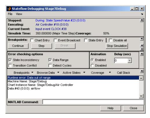
As expected, the error occurs in the during action of SpeedValue because the value of airflow is out of range.
