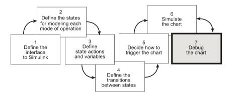
You have entered phase 7 of a basic workflow for building a Stateflow chart: *debugging the chart*. In Chapter 8, "Simulating the Chart", you learned how to use the debugger for setting breakpoints and observing data. In this chapter, you will learn how Stateflow software detects errors and provides diagnostic assistance.
